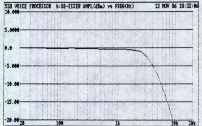
Figure 4.16B Transfer function provided by settings shown at left.
