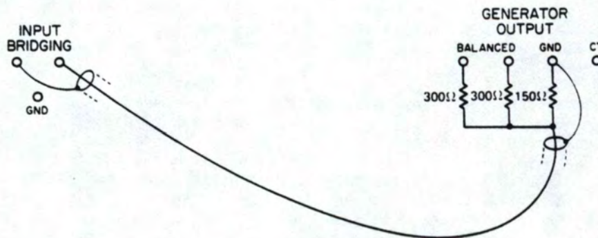
Figure 3-2. Balanced Check Test Setup.
