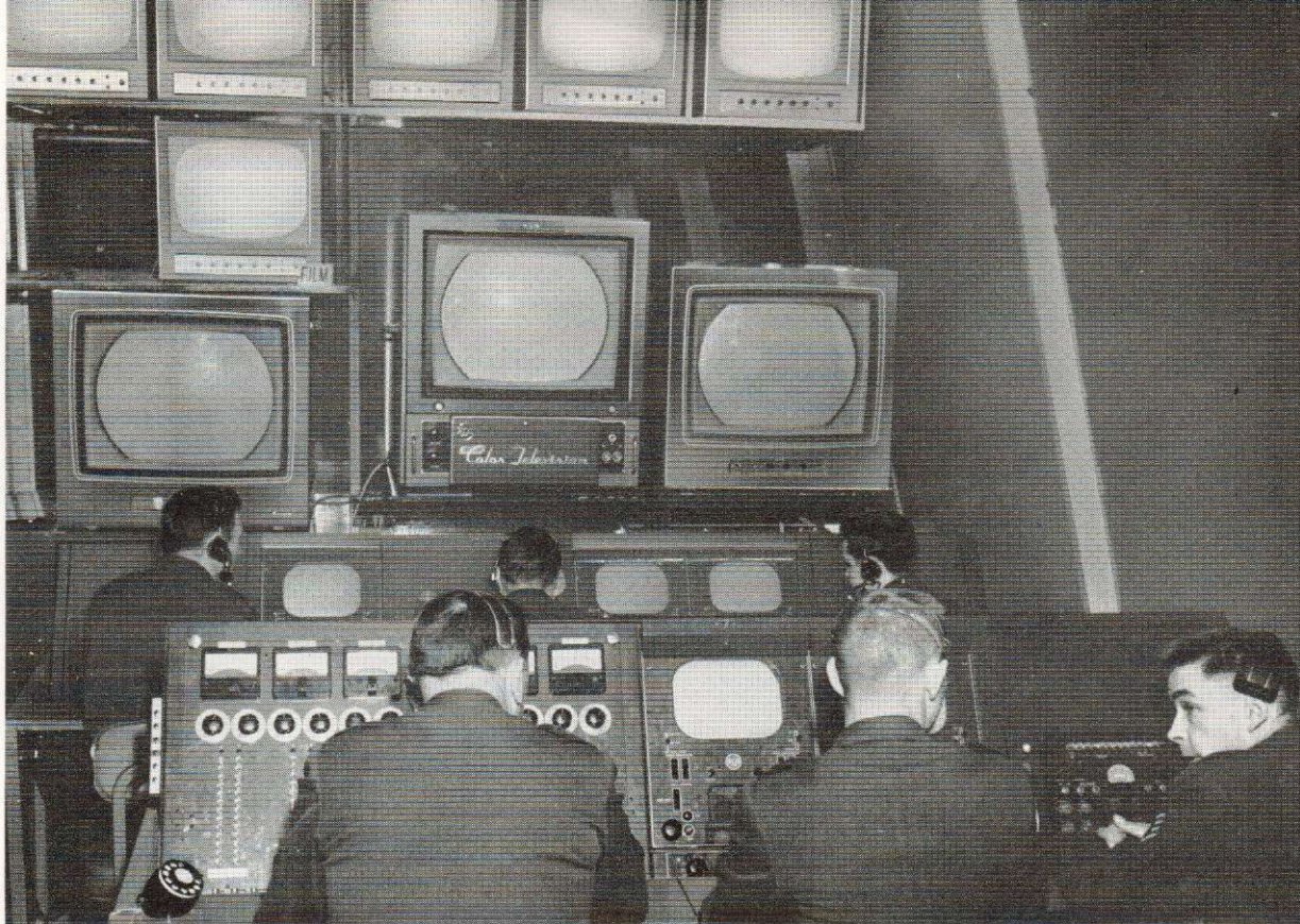
FIG. 9. Here is the well-equipped SAC TV control room. Personnel operating controls are of the Presentation Branch, Control Division, Directorate of Operations. They control cameras, and do the switching.
