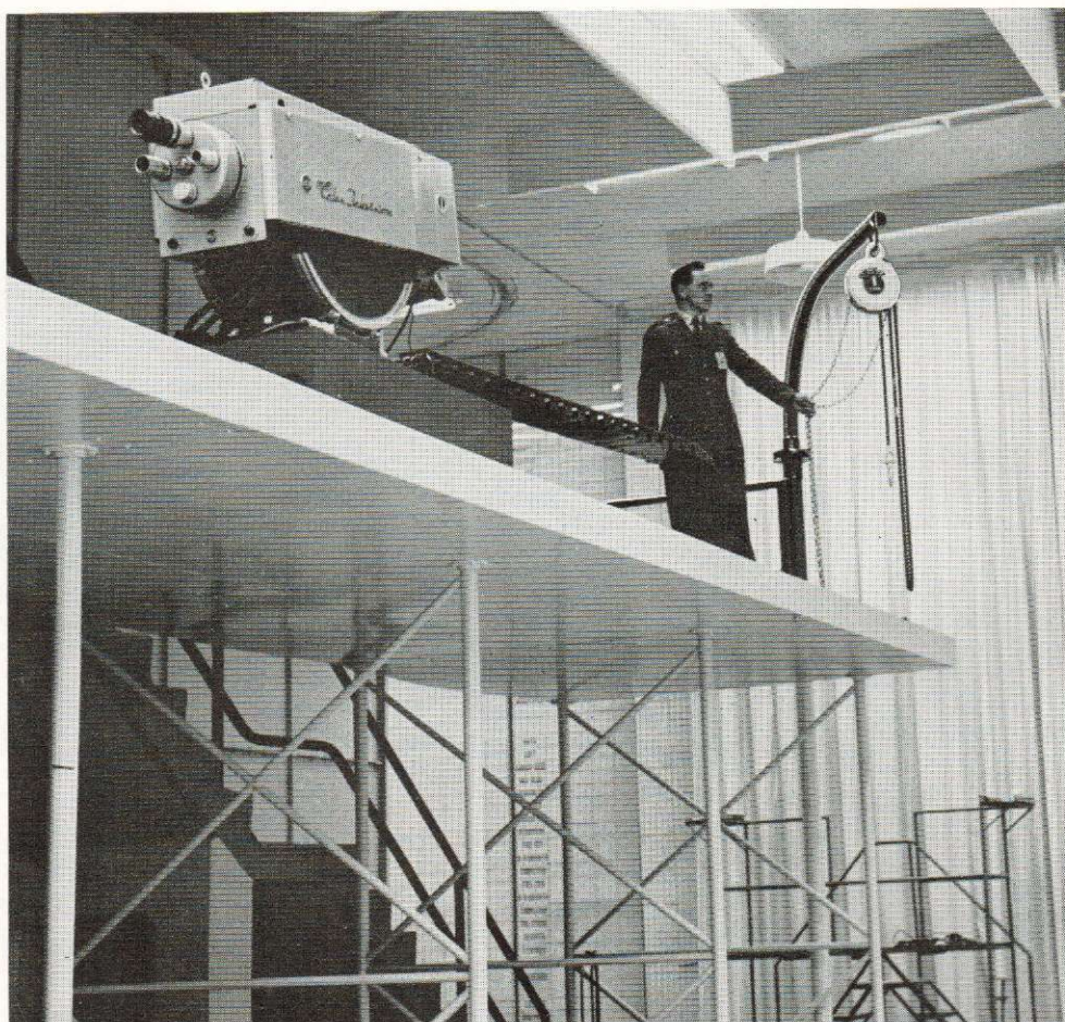
FIG. 18. Maintenance, performed on schedule, keeps SAC TV equipment in top-operating condition. Here Warrant Officer T. G. Ball inspects the hoist, used to convey heavy camera equipment to and from first floor level when major repairs are necessary.
