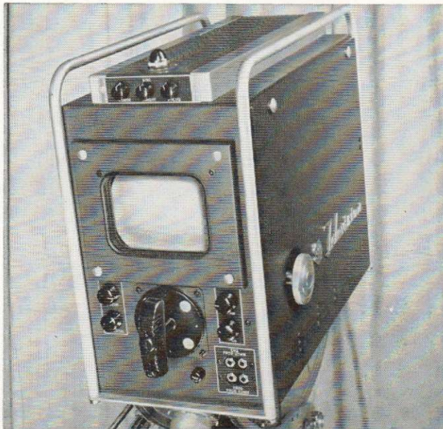
Rear view showing large 7-inch viewfinder and controls.
