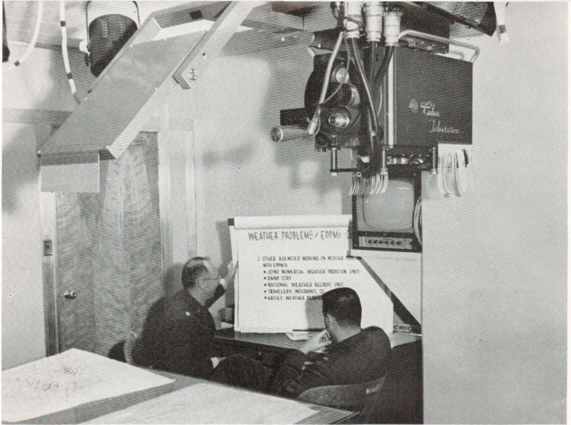
FIG. 6. This 3-vidicon TK-45 Color Camera is located in the Weather Briefing Room on the second floor of the control center. It views weather charts and other data for programming in the SAC color system when needed.
