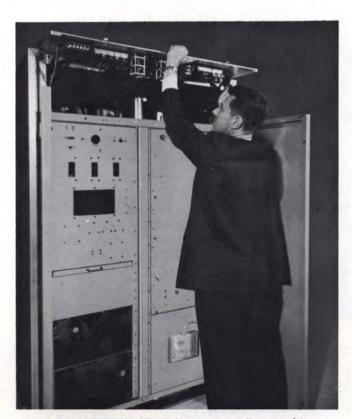
**EASE OF MAINTENANCE**—Full access to all transmitter sections is an important feature in the mechanical design of the BTF-20E.
