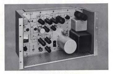
Nine-tube, direct-FM exciter provides unparalleled multiplex performance.
