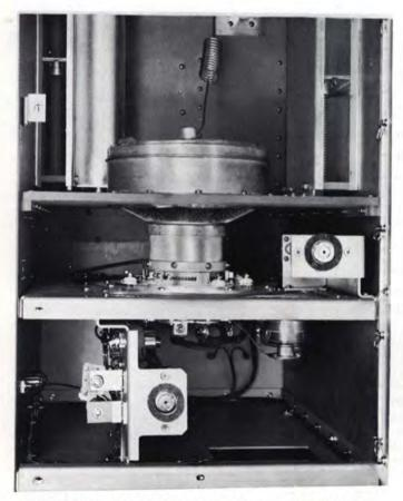
ONLY THREE TUBES BETWEEN EXCITER AND OUTPUT— View showing interior of PA and IPA cabinet with the 4CX15000A ceramic tetrode and two IPA tubes below shelf.
