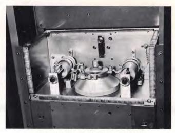
RF cavity with shielded cover removed.
