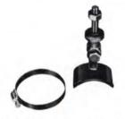
Fixed hanger for single line. Requires mounting hole. Complete with clamp and pivot bolt to compensate for line misalignment.
