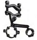
Spring hanger for single line. Complete with clamps and pivot bolt to compensate for line misalignment. Spring must be preloaded at installation.
