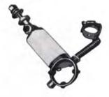
Spring hanger for single line. Mounting hole required. Complete with clamps and pivot bolt to compensate for line misalignment. Spring must be preloaded at installation.
