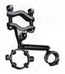
Spring Hanger for single line. Complete with clamps and pivot bolt to compensate for line misalignment. Spring must be preloaded at installation.
