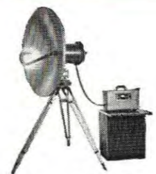
RCA Microwave Relay Transmitter TTR-1A. Transmits the picture signals from field to studio (or from studio to transmitter). It includes a parabolic antenna with hook-shaped wave guide, built-in transmitter, and remote control unit. Matching receiver unit at the station picks up the microwave relay signal.
