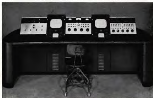
Transmitter Console, Preview Monitor and Switching Turret (right sections)
