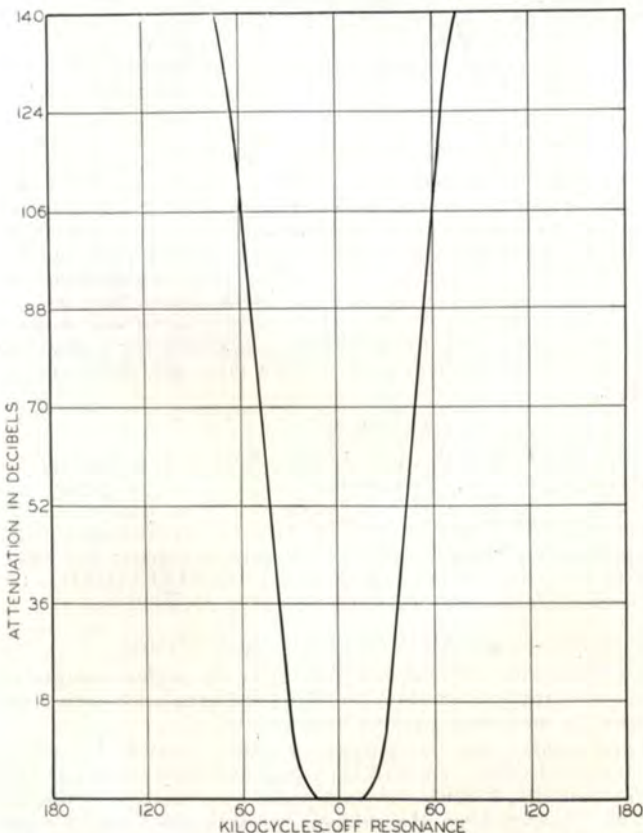
Selectivity curve of the CARFONE. "31 Circuit" Selectivity attenuates adjacent channel signals ( \pm 60 kc) by more than 100 db.
