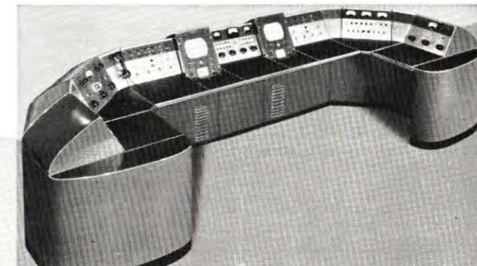
De luxe set-up for combined centralized control . . . AM-FM and TV. Extreme left and right sections are the AM (or FM) transmitter controls. Each includes a transmitter-control, audio-control, and blank wing turret. Center turret controls (for RCA 5-kw TV transmitter) are, left to right: TV power, picture monitor, TV audio, preview monitor, TV program switching.
