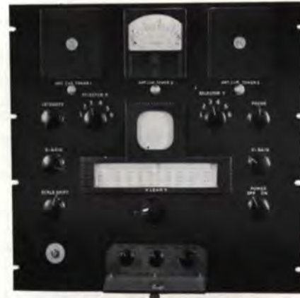
WM-30A Phase Monitor. Blanks in top of panel are to provide for additional meters
