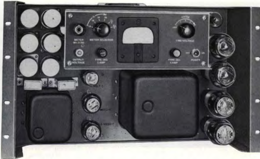
The Regulated Power Supply, MI-26086, as furnished for mounting in a standard rack
