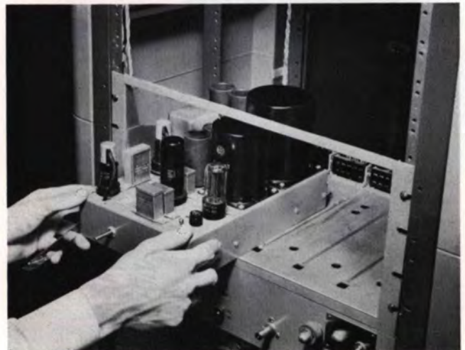
Plug-in amplifier permits quick and easy removal or interchange of units
