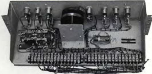
Rear view showing switches, relays and terminal strip.
