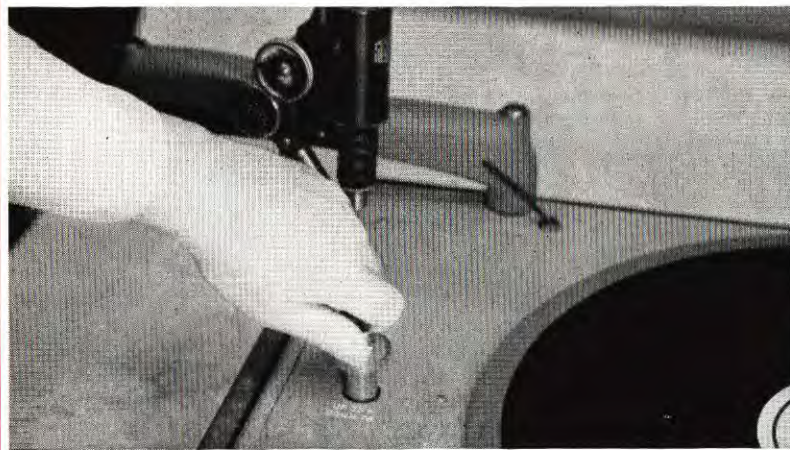
SPEED-CHANGE is simply accomplished by operating the control knob shown here. "UP" is 33 1/3 RPM—"DOWN" is 78 RPM.
