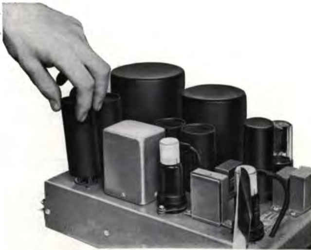
"Plug-in" type electrolytics provide long-life operation and maximum accessibility
