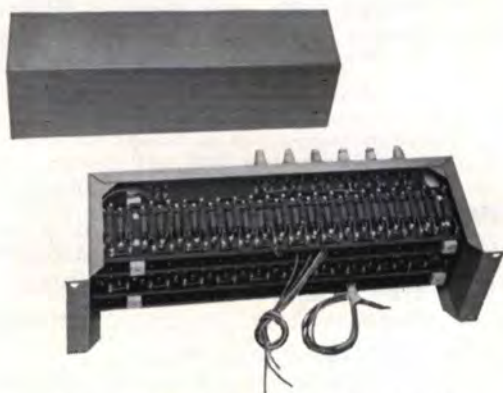
View of Sync Generator Delay Panel shown with protective cover removed
