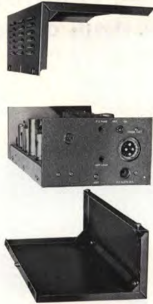
Accordion view showing construction of chassis and covers. Unique construction permits mounting on either right or left side.
