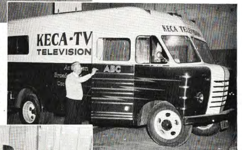
KECA-TV. KECA-TV's television field truck—like many other TV stations—is an RCA "studio on wheels." It is complete with RCA image orthicon cameras, camera tripods, camera control units, on-the-air master monitor, camera switching system, sync generator, microwave relay equipment, power supplies. KECA-TV also uses RCA studio cameras, film equipment, turntables, microphones, and an RCA Superturnstile antenna.
