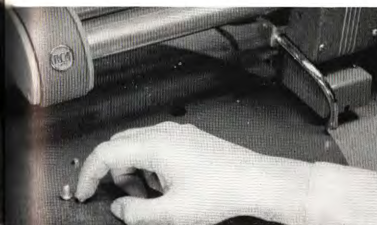
RECORD-DRIVE PIN comes up into position when this plunger-release button is pressed. Pin sinks into platter for records without driving holes.
