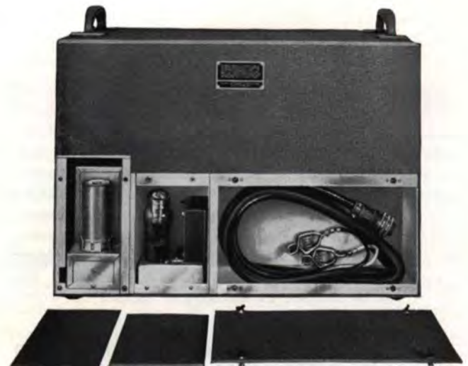
Rear view of WX-1A with cover plates removed. Compartments left to right are: Removable Vibrator Power Supply, Voltage Regulator and Filter, and cable and storage compartment.
