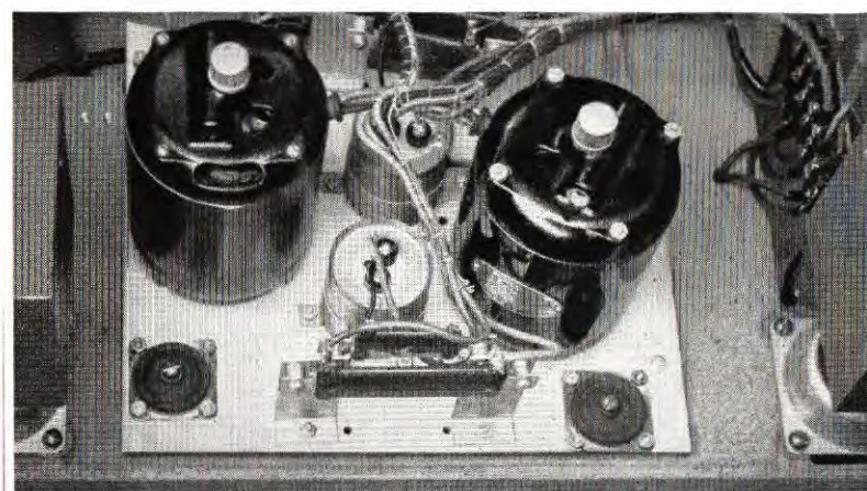
TWO SYNCHRONOUS MOTORS hysteresis type, are coupled to wheels which rim-drive the turntable through sturdy, rubber-idler rollers.
