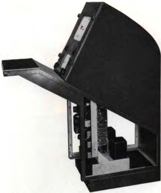
Camera Control Unit showing interior arrangement. This unit is normally housed in the master control console.
