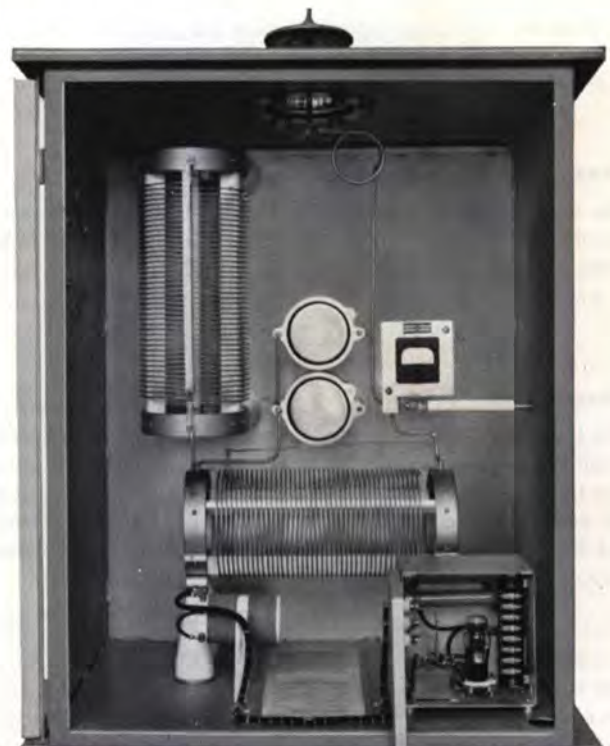
Interior view of BPA-10 with MI-7488A Monitor Rectifier
