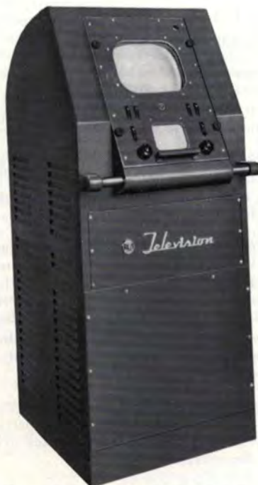
Photo above shows how TM-5A may be mounted in a special housing for portable uses
