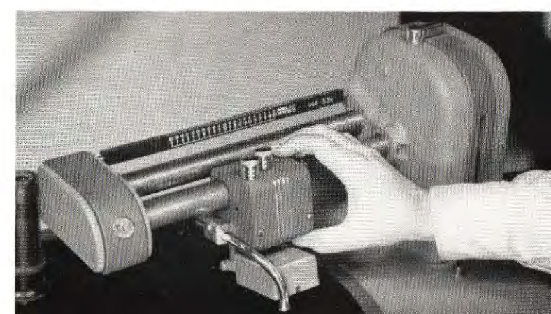
CARRIAGE LEVER is being pressed to allow movement of recorder-head horizontally over the record to desired "cutting" position.
