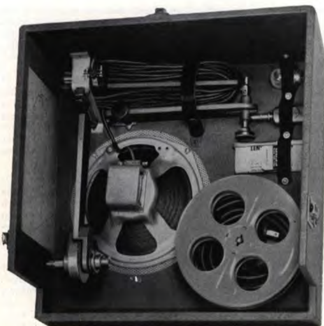
This sturdily built speaker case houses the 8" PM speaker and accessories
