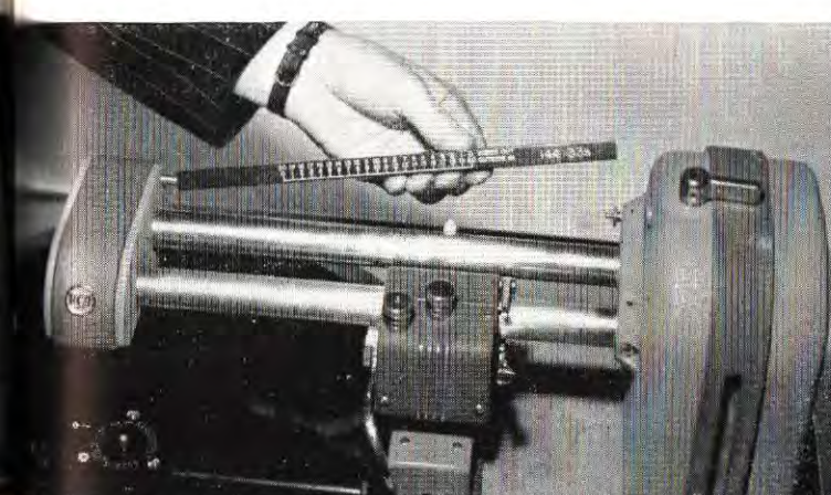
CALIBRATED TIME SCALES for 96, 104, 112, 120, 128, 136, 144 and 152 ("inside-out," "outside-in," at 33 1/3 or 78 rpm are provided. Here, proper scale to agree with "pitch" setting is inserted.
