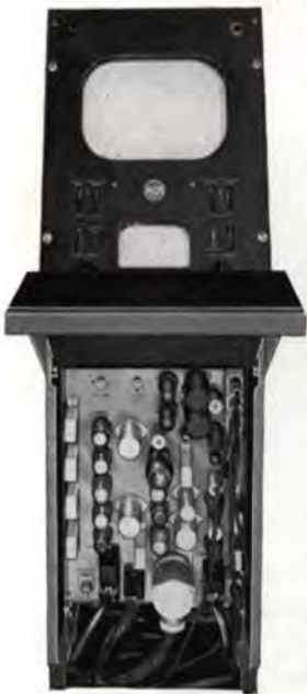
Studio Camera Control Unit consisting of TM-5A Monitor and Camera Control Chassis (MI-26055) mounted in console housing (MI-26266B)
