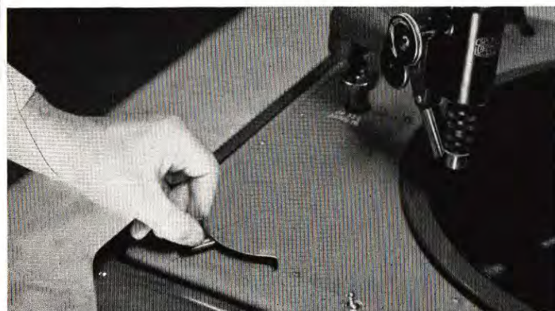
A SINGLE "OFF-ON" lever controls both synchronous turntable drive motors. In "OFF" position, a brake brings turntable to quick stop.
