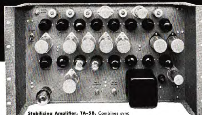
Stabilizing Amplifier, TA-5B. Combines sync and video signals. Corrects defective video signals. Eliminates hum. Corrects low-frequency response. Improves signal-to-noise ratio of sync signals.
