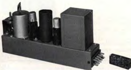
Rear view of BA-11A showing multi-contact, plug-in connection
