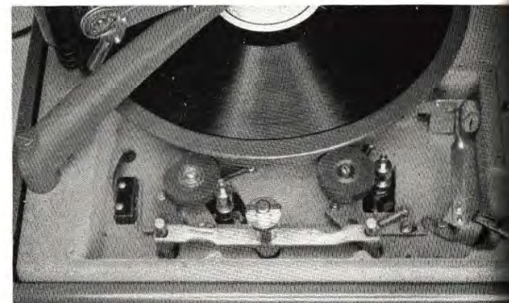
ON-78 RPM —In "ON" position, the brake shoe moves away from turntable rim and rubber idlers are now in active contact with drive wheel and turntable rim.
