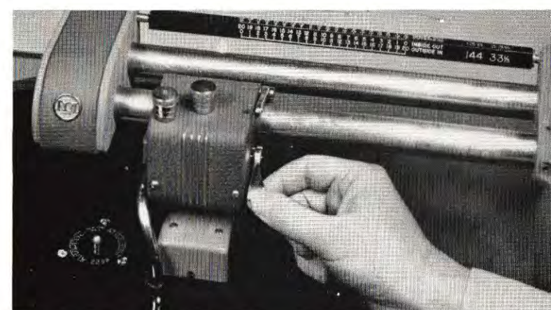
RAISING AND LOWERING the cutter head is easily done by this lever which permits raising the "to rest" position or a gentle lowering to the recording position.
