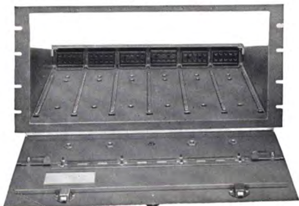
Panel removed showing guide bars and receptacles.
