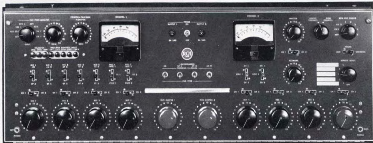
Etched front panel of the BC-6A Consolette showing entire operating facilities.
