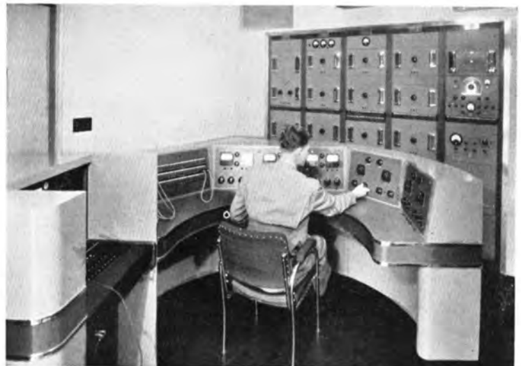
Speech Input Master Control Desk and Racks employed at the Golden Gate Exposition.
