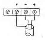
Feed signal to plus and minus terminals with shield tied to ground. The source feeding the console input must have balanced output for this mode.
