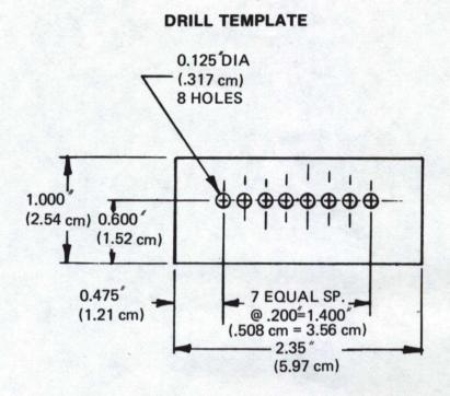
NOTE: We suggest that you measure the diameter of the LED before drilling. The LED you have may be slightly larger or smaller than the hole sizes called out in the drill template.
