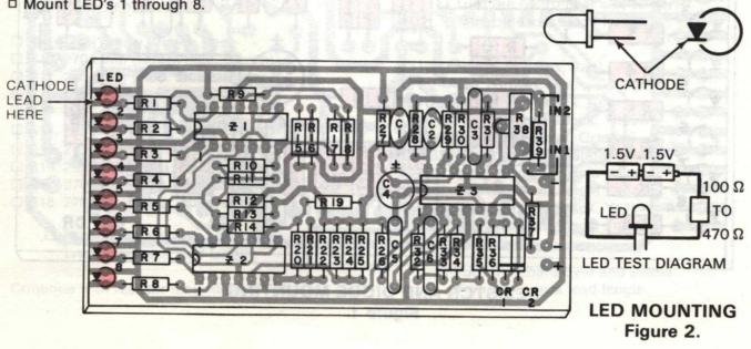
Next install the Integrated Circuits. With any IC, you must take care when handling them. When installing, make sure the leads are straight and that all leads protrude through the holes in the Printed Circuit Board.
