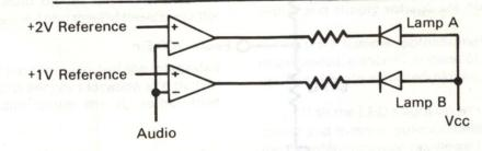
The above illustration shows two comparator stages. Assume that the (+) inputs are connected to a reference voltage source with two taps, one at +1V and one at +2V. The audio voltage may vary from zero volts to +2.5V.
