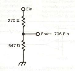
Note that the output voltage (Eout) is almost exactly 3 dB, or a factor of 0.7071 (0.706 to be precise), lower than the input voltage (Ein). The 647 Ohm equivalent-resistor is made up of a 2200 Ohm resistor and a 917 Ohm load.
