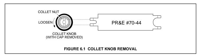
Once the nut is loosened, the collet should release from the shaft. This nut should not need to be removed unless the collet refuses to release.
