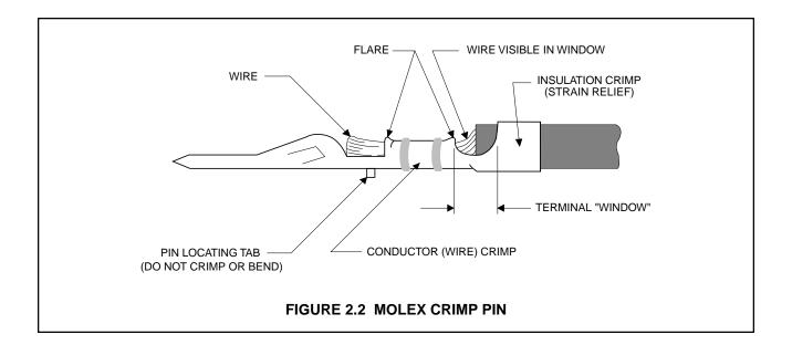
Now place the long ears of the pin into tool notch "A", with the ears pointing toward the letter "A". Crimp the long ears over the insulated section of wire. See Figure 2.2 for an example of a properly crimped Molex pin.
