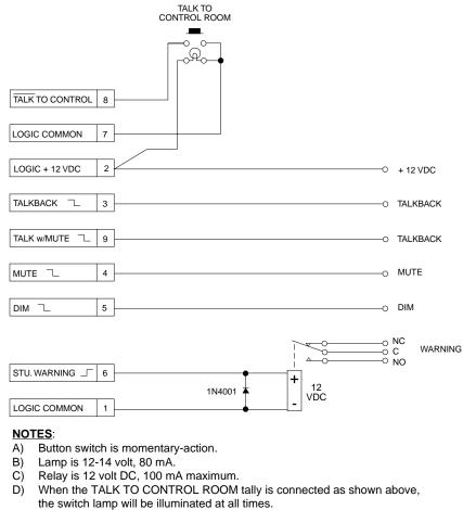
E) The MUTE and DIM outputs are only active when Talkback is taking place via a console Microphone Input Module.
