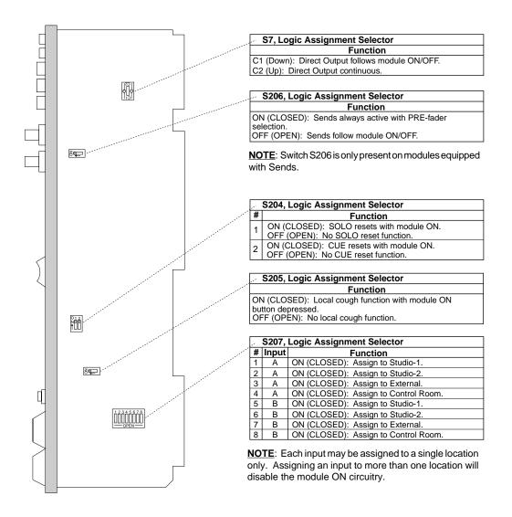
Switch S7 sets whether the module's Direct Output follows the ON/OFF status of the module or has continuous audio output.
