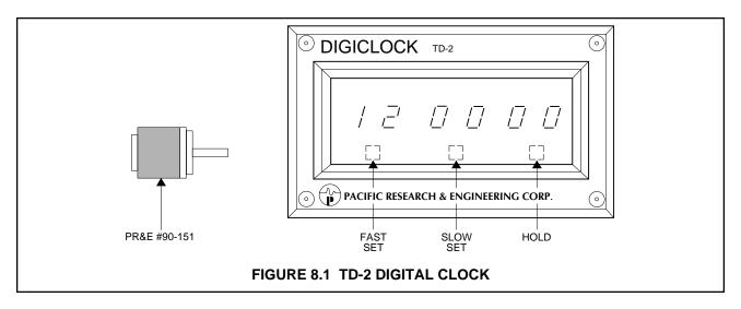
To adjust the clock, place the end of the adjusting magnet against the panel in the appropriate area. Use the FAST SET switch to advance the hours, and the SLOW SET switch to advance the minutes. The HOLD switch will cause the hours, minutes and seconds to stop and hold at their current setting.
