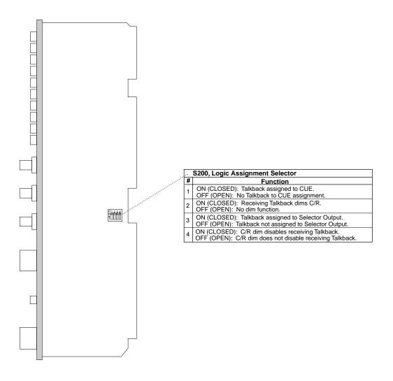
Switch S200-1 allows Talkback to be assigned to the console CUE system. The CUE output is dimmed by 10 dB while Talkback is inserted at unity level.
