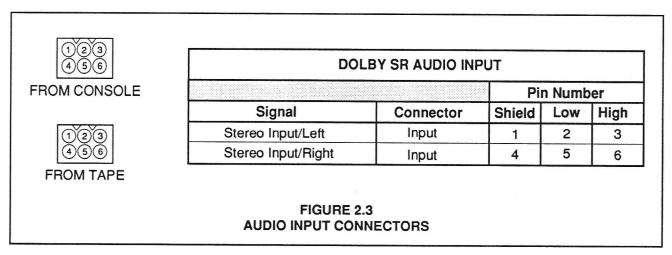
NOTE: A standard connection theme is used throughout most PR&E equipment designs - the use of 3,
