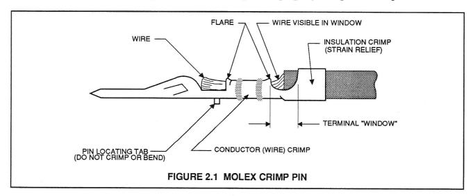
In order to crimp, insert the short ears of the Molex crimp pin into notch "B" of the crimping tool (PR&E #70-3), with the ears pointing toward the letter "B". Insert the wire into the terminal so that the stripped portion is between the short crimp ears, and the insulation is between the long crimp ears. Crimp the short ears.
