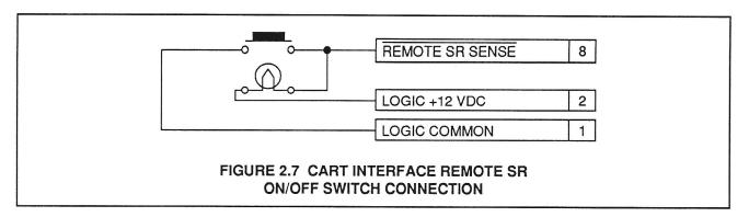
This allows the SR processing function to be controlled remotely by the operator whenever the cart interface module front panel SR MODE switch is in the SENSE position. When using this method of remote control, it it will be necessary to set the internal option switch on the interface module to the "SENSE = ON" position (reference Section 2.9), so that when the switch is engaged SR processing is also engaged.
