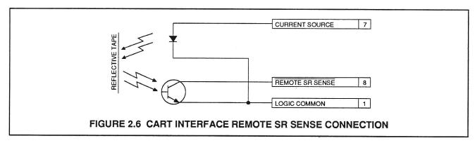
In order to enable the Remote SR Sense function, place the cart interface module's front panel SR MODE switch into the SENSE position. Then, when a cart with a reflective scan tape is installed in the cart machine, the reflective switch will send a signal to the interface module turning SR processing on or off, as determined by the interface module internal option switch described in Section 2.9.
