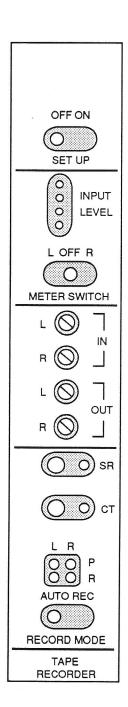
• The SET UP control engages and disengages the Dolby Noise calibration logic of the SR Processing Modules. This switch will be placed to the ON position when playing back Dolby Noise for the purpose of alignment verification, as described in Section 5.4.
