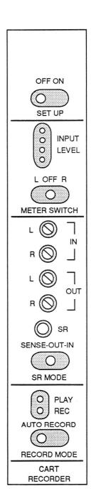
• The SET UP control engages and disengages the Dolby Noise calibration mode of the SR Processing Modules. This switch will be placed in the ON position when playing back Dolby Noise for the purpose of alignment verification, as described in Section 5.4.
