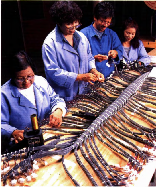
Our system engineers use custom software programs to create the manufacturing plans which are then used by wiring harness assemblers to wire the systems.
