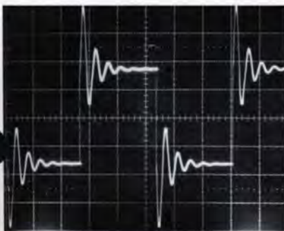
Fig. 5: Output of same equalizer as fig. (2) with 12 dB boost and a "Q" of 3.2. The overshoot is decreased, so we once again raise the gain in the equalizer for the photo. This time, the ringing takes a much longer time to damp out, and would tend to be very audible. The corresponding family of frequency response curves is shown in fig. (11).
