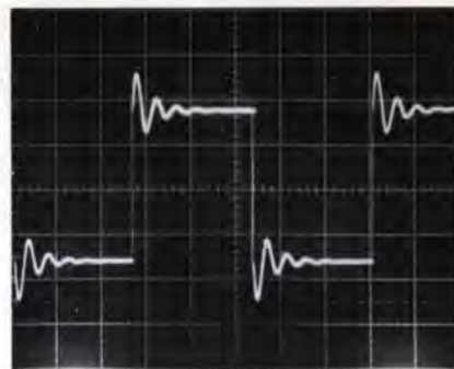
Fig. 6: Output of the same equalizer as fig. (2) with 6 dB boost and a " Q " of 3.2. Because this is a "constant Q " design (like the Orban Parametric Equalizer), the magnitude of the overshoot decreases, but the ringing takes exactly as long to damp out as it does in fig. (5), where 12 dB of boost is used.
