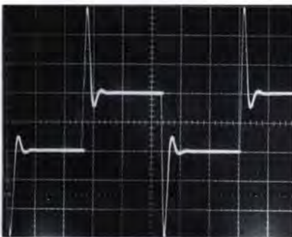
Fig. 4: Output of the same equalizer as fig. (2) with 12 dB boost and a "Q" of 1.0. Once again, we have increased the gain, as the overshoot once again decreases. However, ringing is now visible, although it is rapidly damped out and would not tend to be audible.
