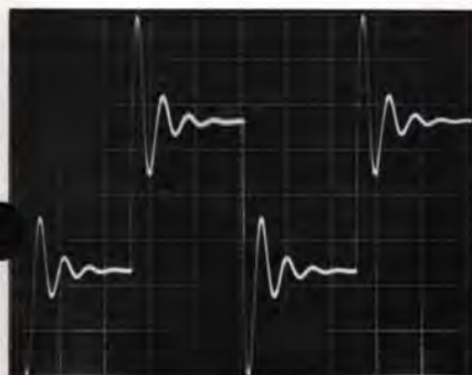
Fig. 13: Square wave response of the reciprocal equalizer of fig. (12) at maximum boost (10 dB). Note the large amount of ringing, and the time necessary to damp the ringing out.
