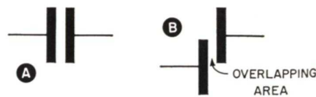
FIG. 4. Only the overlapping areas of the plates affect the capacity of a capacitor.
