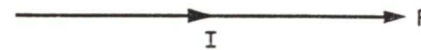
FIG. 28. The voltage across a resistor is in phase with the current, so the vector for the resistor voltage is drawn on top of the current vector.
