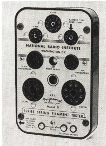
FIG. 17. The NRI Professional filament checker can be used to locate a tube with an open heater in a series string.
