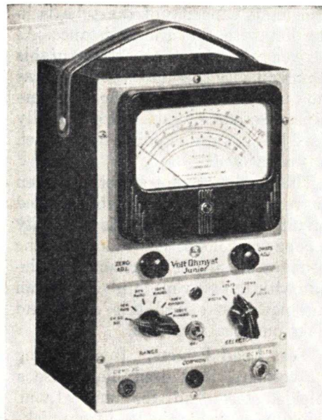
FIG. 9. The RCA-Rider Volt-Ohmyst Jr. is a typical d.c. type v.t.v.m. using the balanced bridge circuit.
