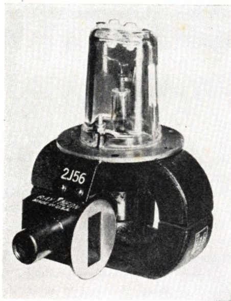
A typical cavity type magnetron.
