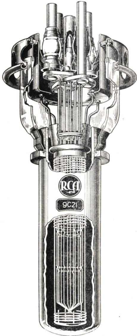
FIG. 4. Cut-away of the 9C21 water-cooled tube.
