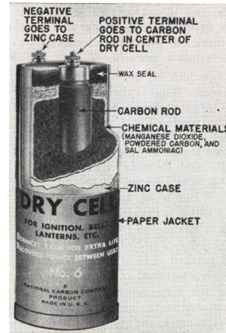
FIG. 1. Construction of a dry cell.
