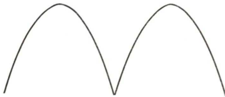
FIG. 29. The output of a full-wave rectifier.
