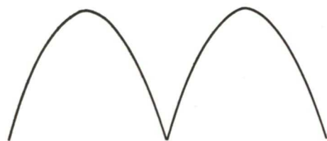
FIG. 16. Output of a simple dc generator.
