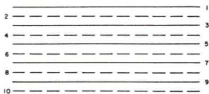
FIG. 24. Example of interlaced scanning. In one field, lines 1, 3, 5, 7, and 9 are scanned, then in the next field, the lines 2, 4, 6, 8, and 10 are scanned. The two fields form one frame of 10 lines.
