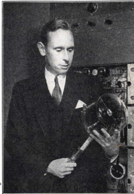
Courtesy Don Lee Broadcasting System The engineer is holding an electronic pickup tube such as is used in television studios. Scanning is accomplished within this tube by electronic means.
