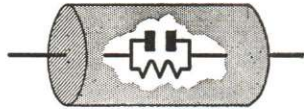
FIG. 18. A practical condenser acts like a perfect condenser in parallel with a high resistance.
