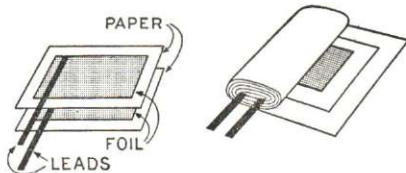
FIG. 6. The "inductive" winding shown here is rarely found in radio, as it can be used only in power packs and audio amplifiers. The non-inductive type shown in Fig. 5 can be used throughout radio receivers or transmitters, so is more commonly found.
