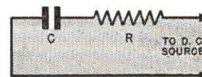
FIG. 22. The condenser charges through the resistor more slowly than it would if the resistor were not used.
