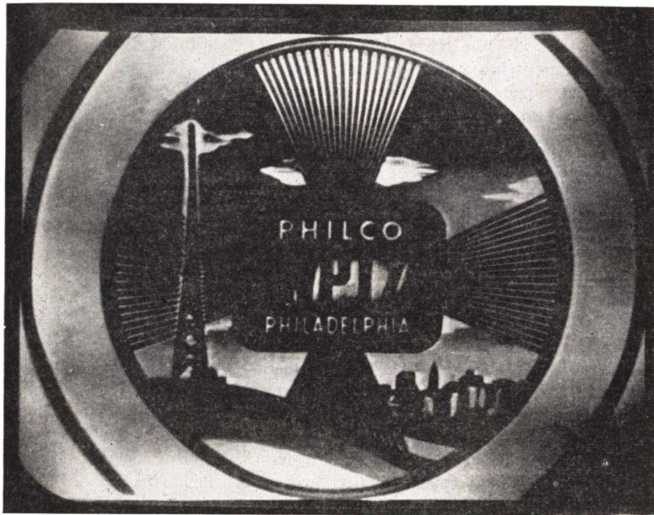
FIG. 8. Excessive contrast (usually caused by setting contrast control somewhat too high).
