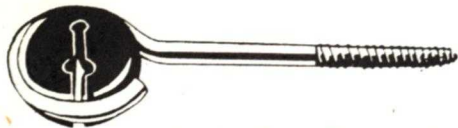
FIG. 31. Stand-off insulator for twin-lead line.
