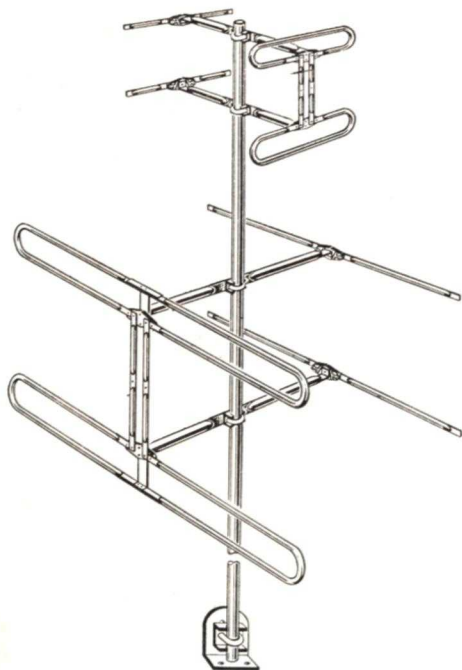
FIG. 18. A fringe-area antenna that can be used to receive stations in both bands at fairly long distances.
