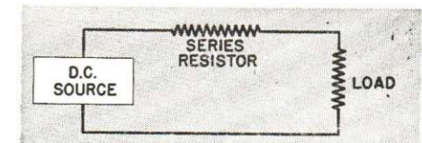
FIG. 5. Basic radio circuit in which the source voltage is too high for the load.
