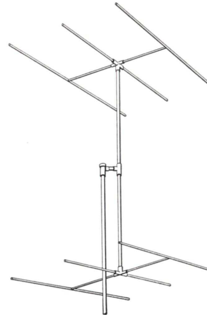
FIG. 31. A stacked array of dipoles, directors, and reflectors.
