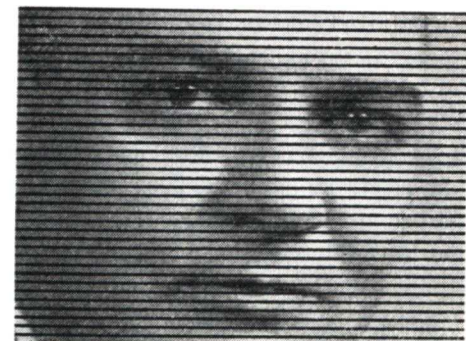
FIG. 3. This enlargement of a section of a TV picture shows that it is made up of a series of lines of varying brightness separated by fine black spaces. (Look at it from 10 feet away and you will see that the lines blend together.)
