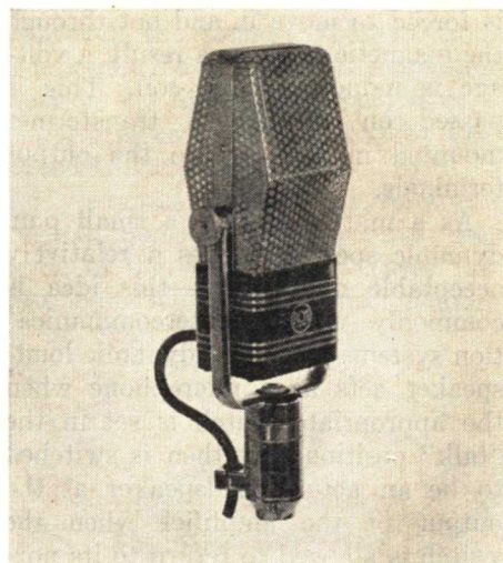
FIG. 10. A typical velocity microphone.
