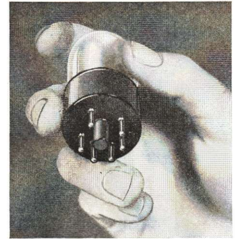
FIG. 8. This is what you see when you remove a 6X5 tube from a receiver and look at its base.
