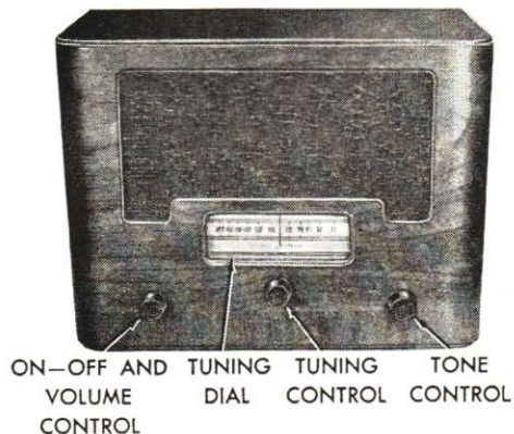
FIG. 3. Front view of the modern superheterodyne receiver used as an example throughout this Lesson.
