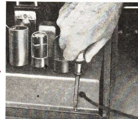
FIG. 5. Using a medium-sized screwdriver to remove the chassis hold-down screws at the back of our superheterodyne receiver.
