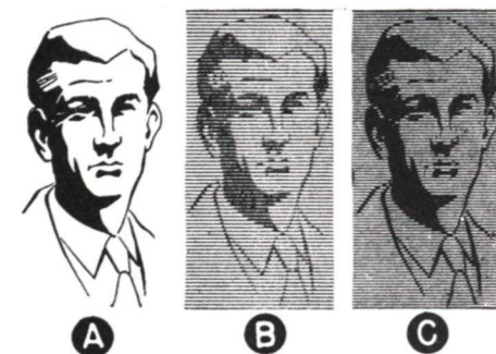
FIG. 2. The drawing at A is reproduced as a series of lines at B and C. Greater detail is obtained by using more lines, as at C.
