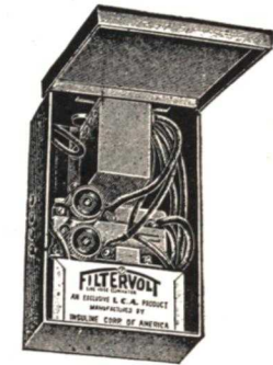
FIG. 6B. Another arrangement of filter units in a steel cut-out box. It is a good practice to place a fuse in series with each condenser, as is done here, for breakdown and short-circuiting of a condenser would otherwise place a direct short across the power line.
