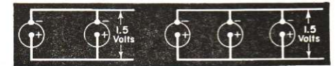
FIG. 20. Parallel connections of dry cells. Remember that when cells are connected together in parallel, the voltage is that of one cell, but the current-furnishing ability is increased.
