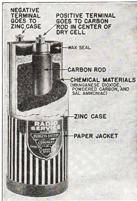
FIG. 17. Construction of a standard dry cell.
