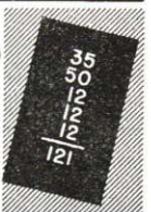
FILAMENTS IN SERIES (UNIVERSAL A.C.-D.C. SET)
