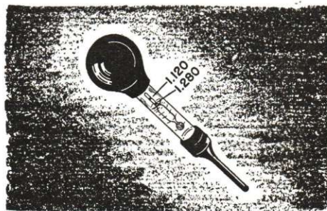
FIG. 23. A hydrometer like this is used to test the condition of each cell in a storage battery. A fully charged battery will give a reading of about 1.280, and a discharged battery will give a reading of about 1.120.
