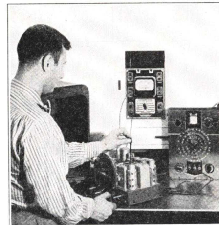
Alignment requires a signal generator and an output meter. Separate instruments, as shown here, or a combination multimeter-signal generator can be used. The signal generator furnishes a signal of known frequency and controllable output. The adjustments are made for maximum indication on the output meter. A simple procedure, yet it is vital to the radio performance that the proper steps be followed.
