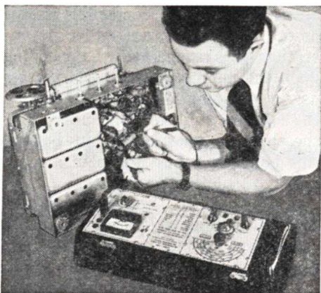
In a case of distortion, effect-to-cause reasoning has led this Radiotrician to check the voltage across a grid resistor. By locating the coupling condenser, this measurement can be made between the chassis and the end of the condenser which connects to the grid of the next stage, as shown here.
