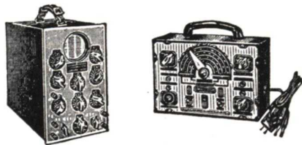
A typical cathode ray oscilloscope and a signal generator.
