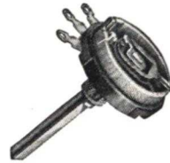
Volume control potentiometers should be replaced when they cause noisy operation.
