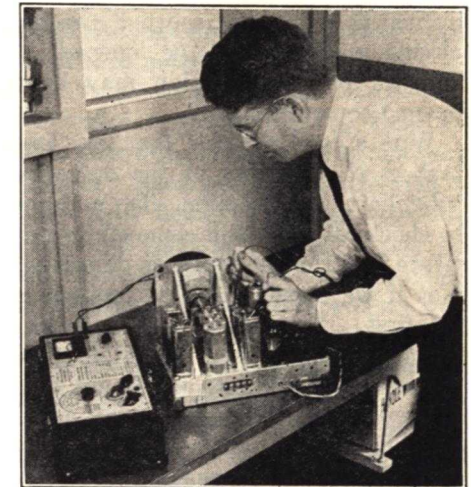
Making a continuity test between the top caps of two tubes on the Philco model 38-7 receiver, using the multimeter section of a combination signal generator and multimeter.
