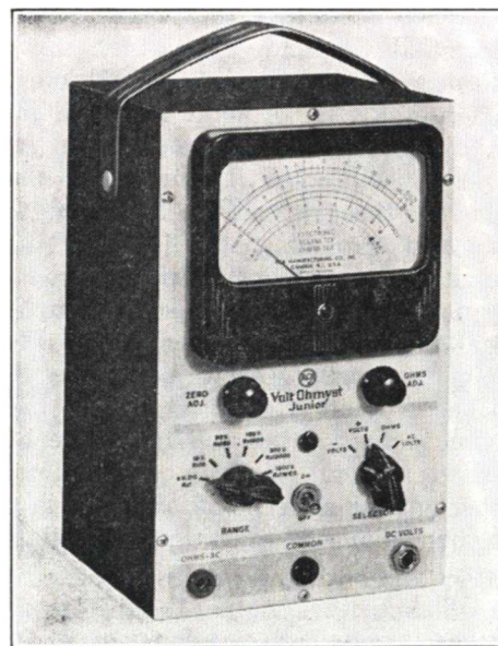
FIG. 11. The RCA-Rider Volt-Ohmyst Jr. is a typical d.c. type v.t.v.m. using the balanced bridge circuit.
