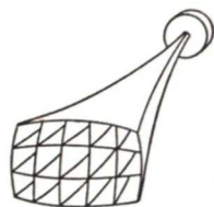
FIG. 19. Horn loudspeakers designed for use as tweeters are often divided into sections as shown above in order to spread out high-frequency sounds.
