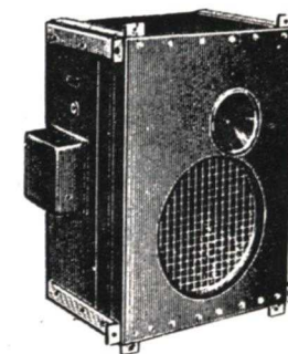
FIG. 28. A large dynamic cone loudspeaker (woofer) and a horn type tweeter are here mounted on a single box baffle to give uniform response over a wide range of audio frequencies. The inside of the box is lined with sound-absorbing material to prevent standing waves.
