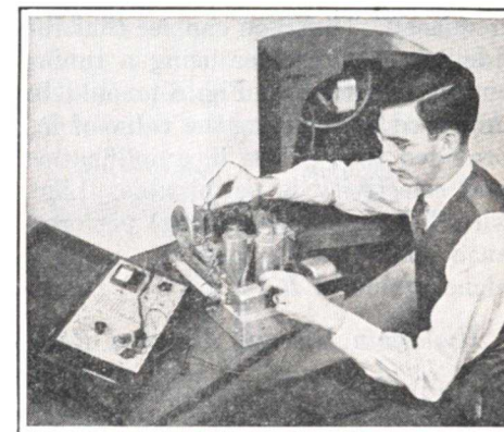
All-wave superheterodyne receiver being aligned for peak response. An R.F. signal generator and an output meter are the only instruments needed. The output of the R.F. signal generator section is fed into the receiver, and the multimeter section is used as an output meter.
