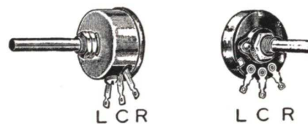
Fig. 17. Two representative manual volume control potentiometers. In each case two nuts are provided on the threaded tubular projection of the housing (through which the shaft runs) to permit clamping the control to a receiver chassis. Only a single mounting hole is needed.
