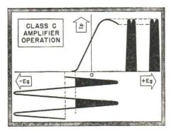
FIG. 7. In class C operation, even less than half of the incoming signal is used to produce plate current pulses.
