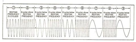
' FIG. 23. A fundamental representation of a frequency-modulated wave.
