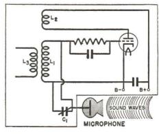
FIG. 24. This simple circuit shows one possible way of frequency-modulating an oscillator. Of course, practical circuits are far more complex.
