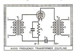
FIG. 19. Transformer coupling is employed when high gain is desired, as you will learn later.
