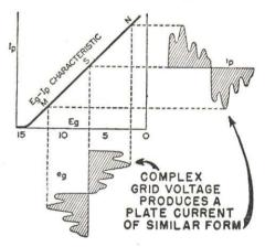
FIG. 5. The signal currents handled by most radio and television tubes have irregular wave forms much like that shown here for eg. It can be proven by mathematics, however, that any wave, no matter how complicated, can be broken up into a number of simple sine waves. We can simplify our work by considering only sine-wave signals, for we know that radio circuits will behave the same for a particular sine wave as they do for this component of a complex wave.
