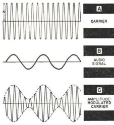
FIG. 22. When the carrier at A is modulated by the audio signal, B, the result can be represented by C.
