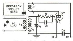
FIG. 21. A basic oscillator circuit.
