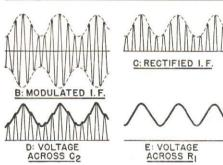
FIG. 27. The diode is also commonly used as a demodulator.
