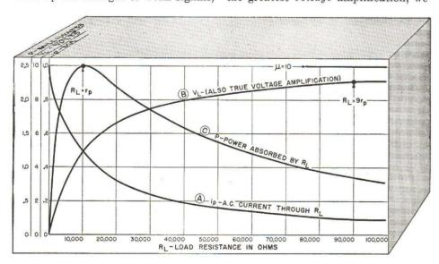
FIG. 14. These curves show the effect that various load values have on the plate current, load voltage, and power output. The higher the load value the greater the VOLTAGE gain. The load should equal the source impedance for greatest POWER output.
