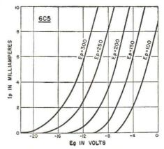
FIG. 9. A family of characteristic curves. bination of the other two).
