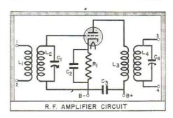
FIG. 20. This tuned amplifier circuit is known as a t.r.f. stage.
