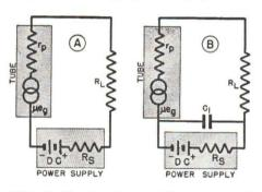
FIG. 15. How the effects of the power supply resistance are eliminated by a by-pass condenser.
