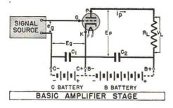
FIG. 13. By inserting the proper signal source, the proper load value, and the correct operating voltages, this basic circuit can be made to fit ANY AMPLIFIER USE!
