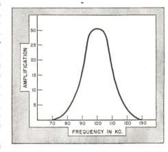
FIG. 28. The response curve of a resonant circuit.
