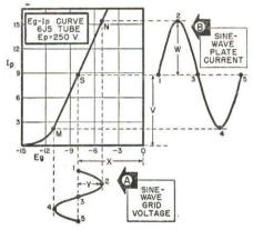
FIG. 4. The Eg-Ip curve for a 6J5 tube, with a plate voltage of 250 volts. It is assumed that the proper filament voltage is applied to the
