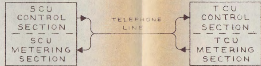
B) WIRE REMOTE CONTROL SYSTEM
