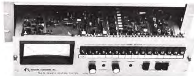
Front View, slide-out drawer partially extended, Studio Unit. Total access is afforded to active circuitry.
