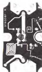
Micro-strip techniques are used where applicable in the PCL-505 Transmitter and Receiver. Shown is a module from the PCL-505 Receiver.
