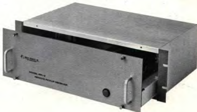
Note slide-out drawer construction of RPL-2R Receiver giving complete access from the front panel.
