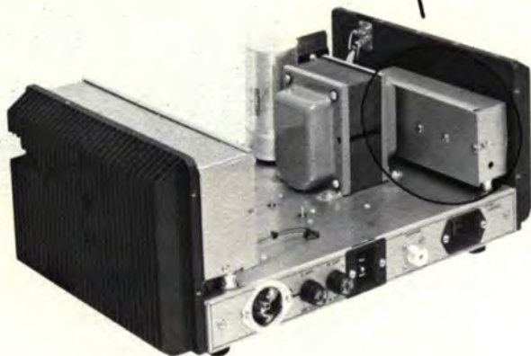
Rear of RPL-2T Transmitter with top cover removed showing varactor tripler assembly. 160 MHz RF final amplifier is mounted on heat sink to left.
