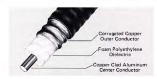
Cablewave Systems Foam Wellflex coaxial cables offer a combination of remarkable flexibility, high strength, and superior electrical performance. The designs include a copper clad aluminum center conductor, low-loss cellular polyethylene foam dielectric, corrugated copper outer conductor and a protective black polyethylene jacket. Foam Wellflex is used extensively in communications and electronic systems in the HF, VHF, UHF and microwave frequency bands.
