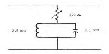
This equalizer is designed to maintain good response out to about 8kHz. This is accomplished by adding mid-band attenuation to bring down the mid-band response to equal that of the high end. This means that all passive equalizers, of necessity, increase overall line losses. Be sure the equipment on the other end of your audio line has the reserve gain to be able to work with the added loss.
