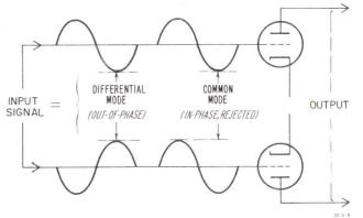
Figure 1-7. Differential Amplifier Input
