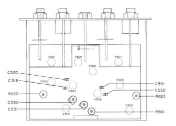
Figure 3-1. Bottom View of Dual Trace Amplifier
