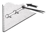
2. Using a small awl, carefully clean inside of hole left by old part.
