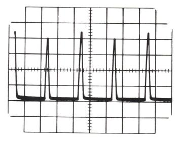
Figure 3-2. Chopped Blanking Waveshape
