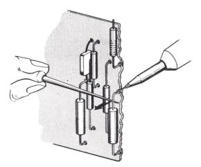
1. Apply heat sparingly to lead of part to be replaced. Remove part from card as iron heats the lead.
