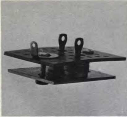
Figure 16.7(a) Dual Diode Mounting ( \theta_{c-s}=1.2-2.2^{\circ}\text{C}/\text{watt} )
