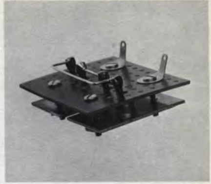
Figure 16.7(b) Full Wave Bridge Using A44 and A45 Dual Diode Sections
