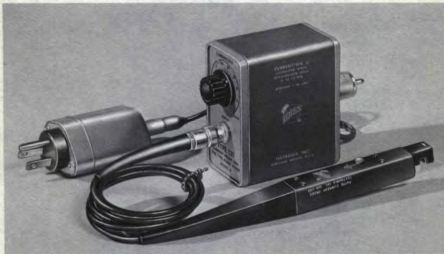
Figure 9.5.1 Current Probe and Amplifier
