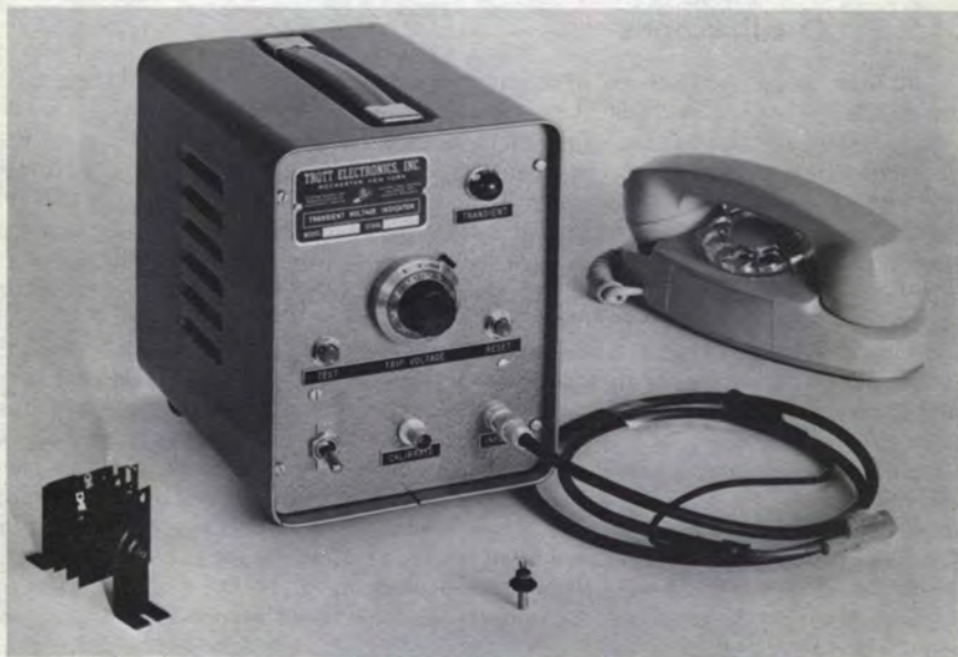
Figure 14.9 Transient Voltage Indicator
