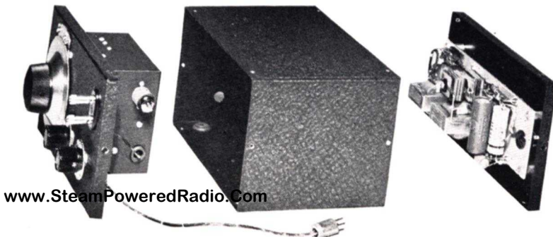
Fig. 5. Disassembled View of the Frequency Standard and Power Supply
