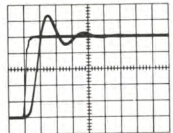
TRANSIENT RESPONSE (Volts: 10mV/Div, Time: 100ns/Div)
