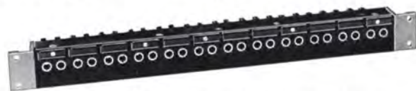
Above, PJ-343 jack panel has 24 jacks (12 pairs). Size: 1 3/4" x 19". Does not require jack mat. End brackets for rack mounting supplied.
