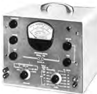
Model 410 Distortion Meter
