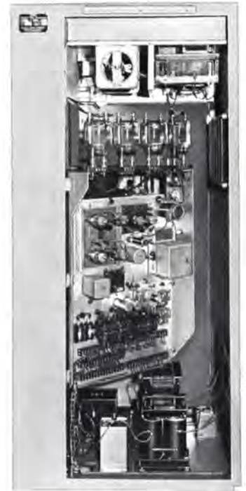
Rear view of the BC-1G transmitter with vertical shelf assembly swung out.
